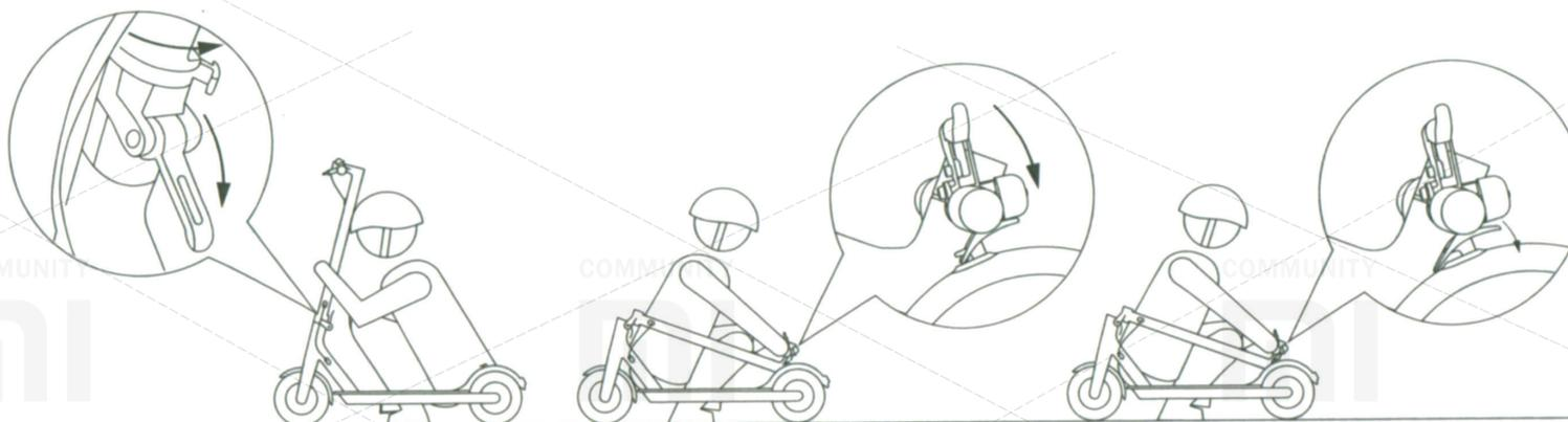
Make sure, that the vehicle is off. Loosen a lock lever and lower a steering rack. Adding a steering rack in a horizontal position and secure it by inserting a hook through a special ring, which is located on the rear wheel mudguard. To assemble the scooter, disconnect a steering rack lock from a hook of a mudguard, and then lift it into a vertical position and lock a lever.
