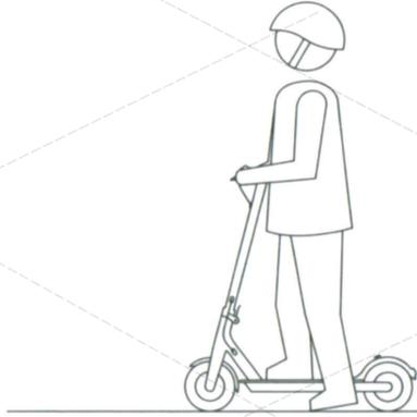
Only when both feet stand on the scooter platform, you can press the speed knob (press the knob at minimum possible scooter speed of 5km/h);
