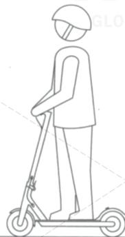
3. When the turns it's necessary to slightly move a body's center of gravity in the right direction, and turn the steering wheel slowly.
